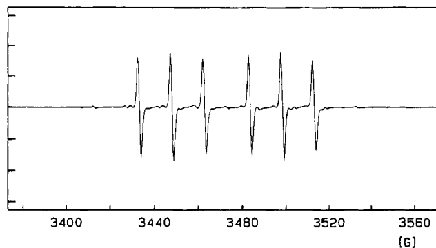
Figure 1. EPR spectrum of the hydroxymethyl adduct of DEP-DMPO in water. EPR conditions: microwave power = 19.9 mW, receiver gain = 1 \times 10^4 , modulation frequency = 100.0 kHz, modulation amplitude = 0.53 G, sweep time = 84 s, scale = 17, center field = 3473.0 G, and sweep width = 200.0 G; spin adduct from photolysis of the solution of DEP-DMPO (0.01M) and 12.5 vol % methanol in 1% hydrogen peroxide.
